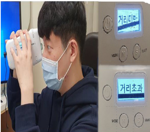
Figure 1. Self-intraocular pressure check using Tono-i tonometer. Different colors are shown according to distance between central cornea and Tono-I tonometer (> 6.5 mm: blue, 5.5-6.5 mm: green, < 5.5 mm: red). Also, the distance is displayed on monitoring board of Tono-i tonometer.
